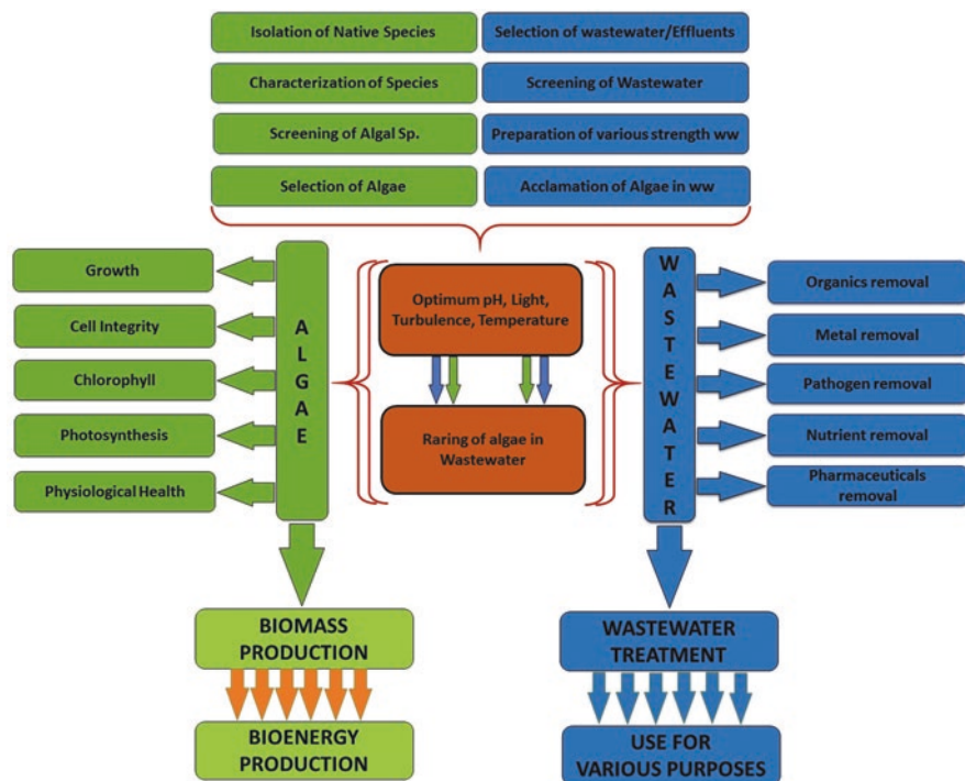
Fig. 18.1 A general overview of algal technologies for wastewater treatment and biomass production for biofuels
