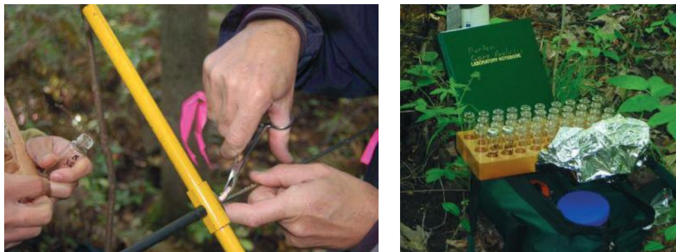
Core samples of trees are taken with a standard arborist's tree coring device and brought back to the lab in vials for analysis. The samples are analyzed to determine if contaminants are present in the tree (Burken, 2014).
