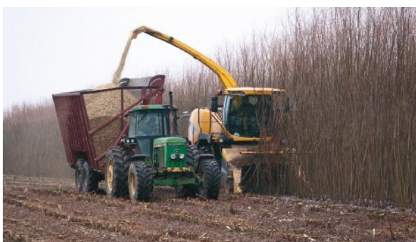
Four-year-old willow biomass crops being harvested with a New Holland forage harvester and coppice header. This system cuts and chips the willow biomass in a single pass (Volk, SUNY ESF, 2014).
