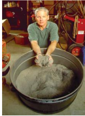
Above-ground plant parts were harvested and incinerated into an ash, ready to be used in the nickel smelting process (Dr. Scott Angle pictured).
